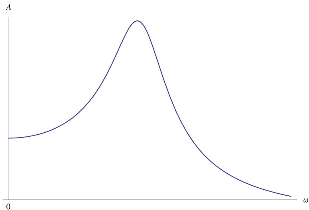
Since the damping is low, the peak of the curve is very close to the natural frequency of  $9.0 \text{ rad s}^{-1}$ . The original frequency was  $6.0 \text{ rad s}^{-1}$  and now it is  $3.0 \text{ rad s}^{-1}$ . So, we have moved further to the left and hence the amplitude is smaller. This means we get the curve in red for the new displacement:
